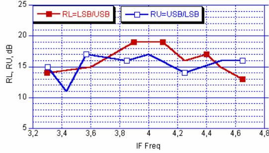
Figure 11 An example of sideband separation ratios as a function of the IF frequency. The plot is obtained for a single LO frequency and by sweeping the CW source along the RF sidebands in the case of IF 3.4-4.6 GHz.
