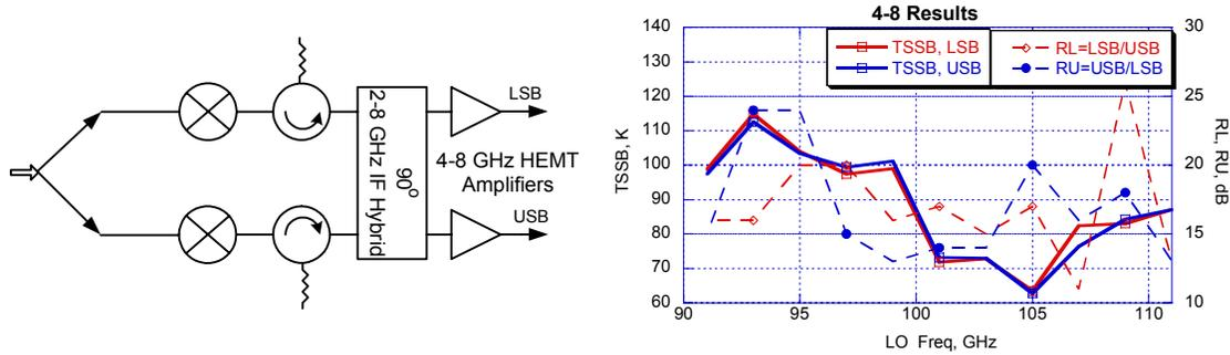
Figure 12 Measured SSB equivalent noise temperature  $T_{SSB}$  – solid lines, and sideband suppression ratios  $R_U$ ,  $R_L$ -dashed lines vs. LO frequency, (equivalent to RF band of 85-117GHz with 6 GHz IF center frequency). IF band is 4-8 GHz and the IF hybrid is in front of the amplifiers.
