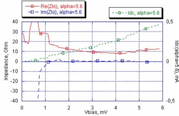
Figure 4 The complex large-signal impedance vs. bias voltage of the SIS-load junction pumped with LO power 15 dB higher than the optimum mixer-junction power ( $\alpha=5.6$  at every bias point). The figure shows also the straighten  $I_{dc}$ .
