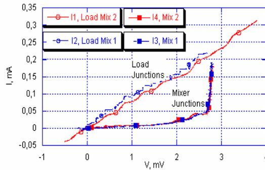
Figure 6 Junctions' I-V curves in the presence of LO power. The mixer junctions are pumped with optimum power for best sensitivity, while load junctions are over pumped being exposed to 15 dB higher power. The pairs of I-V curves show excellent symmetry giving good prospects for high degree of sideband separation.
