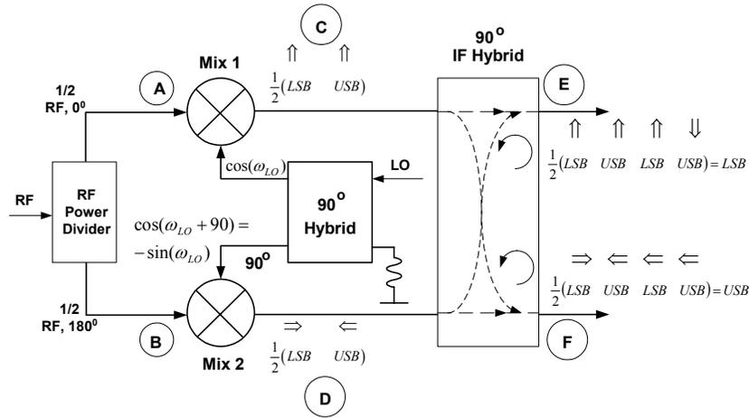
Figure 1 Block diagram of the 2SB mixer. Sideband separation is achieved by using a quadrature scheme where two identical mixer junctions are pumped by a local oscillator (LO) with 90° phase difference. To illustrate the sideband cancellation, the relative phases of the sideband signals are shown at different points of the mixer. USB and LSB stand for Upper and Lower Side Band respectively. The RF power divider is a 3-port structure, which does not contain resistive terminations.
