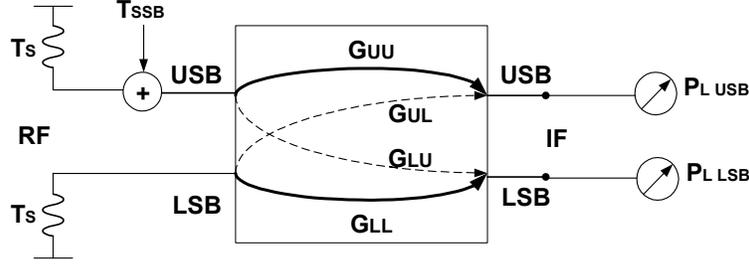
Figure 8 The sideband separating mixer characterized by its SSB equivalent noise temperature. The mixer noise temperature  $T_{SSB}$  is contributed to only one of the sidebands.
