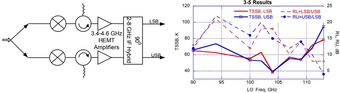
Figure 10 Measured SSB equivalent noise temperature  $T_{SSB}$  – solid lines, and sideband suppression ratios  $R_U$ ,  $R_L$  -dashed lines vs. LO frequency, (equivalent to RF band of 86-118GHz with 4 GHz IF center frequency). IF band is 3.4-4.6 GHz and the IF hybrid follows the amplifiers.
