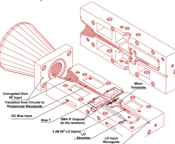
Figure 2 Layout of the sideband separating mixer. The mixer block consists of two identical parts dividing symmetrically all waveguide structures. Waveguide cross-section is 1.2 / 2.4 mm.
