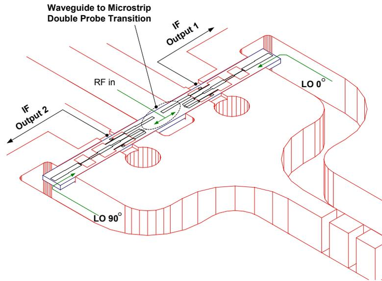
Figure 3 The mixer substrate penetrates 3 waveguides in the mixer block. The divided LO power is introduced at the ends of the substrate while the RF power is coupled to the substrate in the middle and divided between the two mixer junctions by the waveguide to microstrip double probe transition. The mixer substrate is a Z cut crystal quartz with dimensions 0.7 / 8.74 / 0.15mm (W/L/H). The substrate size is chosen such that it does not allow waveguide modes inside the substrate channel.
