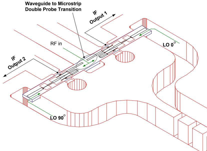
**Figure 4** The mixer substrate coupled to the waveguides. The divided LO power is introduced at the ends of the substrate while the RF power is coupled to the substrate in the middle and divided between the two mixer junctions by the waveguide to microstrip double probe transition. The mixer substrate is a Z cut crystal quartz with dimensions 0.7/8.74/0.15mm (W/L/H). The substrate size is chosen such that it does not allow waveguide modes inside the substrate channel.
