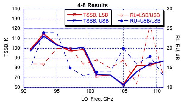
**Figure 8** Measured SSB equivalent noise temperature  $T_{SSB}$  – solid lines, and sideband suppression ratios  $R_U$ ,  $R_L$ -dashed lines vs. LO frequency, (equivalent to RF band of 85-117GHz with 6 GHz IF center frequency). IF band is 4-8 GHz and the IF hybrid is in front of the amplifiers.
