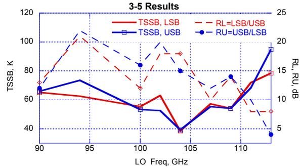
**Figure 7** Measured SSB equivalent noise temperature  $T_{SSB}$  – solid lines, and sideband suppression ratios  $R_U$ ,  $R_L$ -dashed lines vs. LO frequency, (equivalent to RF band of 86-118GHz with 4 GHz IF center frequency). IF band is 3.4-4.6 GHz and the IF hybrid follows the amplifiers.
