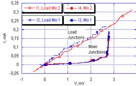
**Figure 6** Junctions I-V curves in presence of LO power. The mixer junctions are pumped with optimum power for best sensitivity, while load junctions are over pumped being exposed to 15 dB higher power. The pairs of I-V curves show excellent symmetry giving good prospects for high degree of sideband separation.
