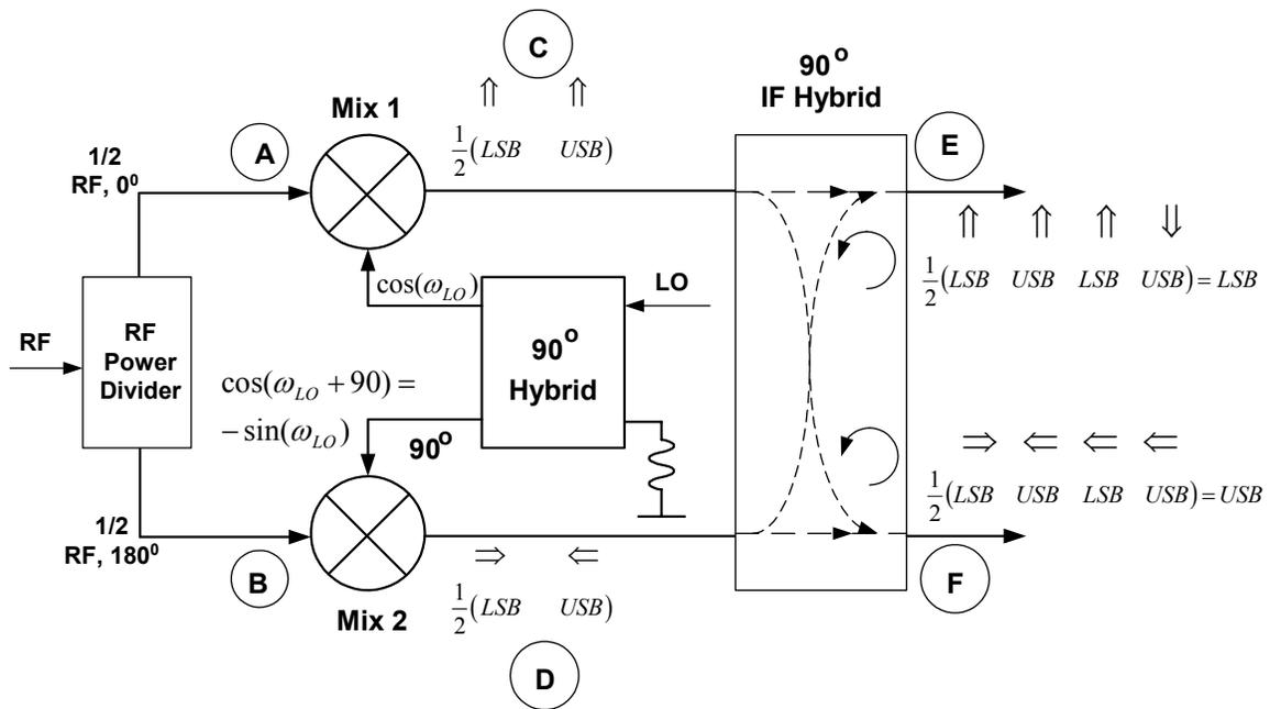
**Figure 2** Block diagram of the suggested sideband separating mixer. To illustrate the sideband cancellation, the relative phases of the sideband signals at IF are shown at different points of the mixer. USB and LSB stand for Upper and Lower Side Band respectively.
