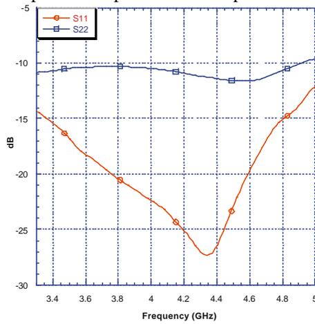
Figure 10. Measured input (solid line) and output (dashed line) reflection coefficient.
