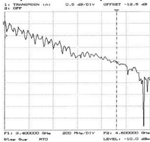
Figure 11 The cable slope before the equalization.
