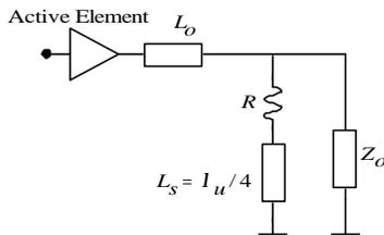
Figure 6. Introducing a slope over the gain of an active element.
