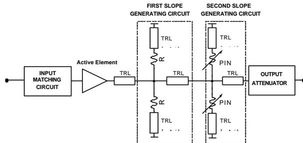
Figure 7 The AEQ block diagram.
