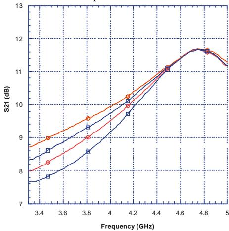
Figure 9 Measured gain of the AEQ for four values of the PIN diode resistance.
