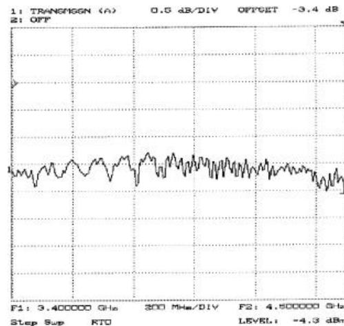
Figure 12 The compensated cable slope.
