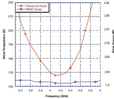
Figure 5 Amplifier's measured noise and the producer specified gain block noise.
