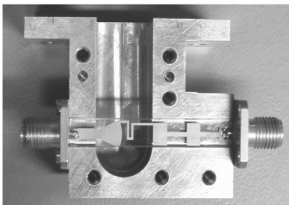
a) Photograph of the split part of the X-band transition. Split-block techniques is used, cylindrical backshort is done to facilitate fabrication at high frequencies.
