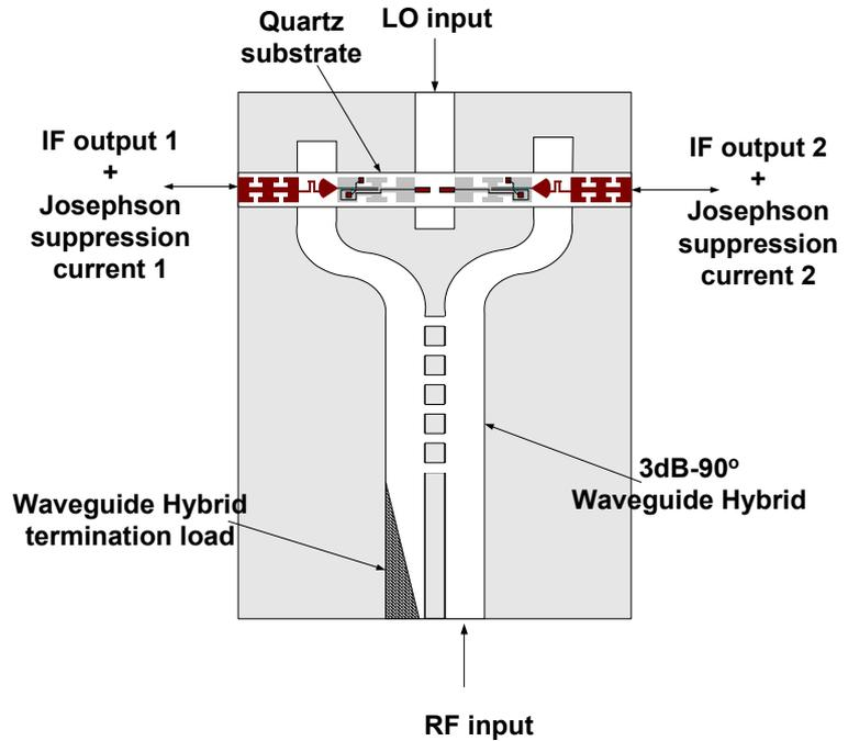
Fig. 2: 2SB mixer for 345 GHz
