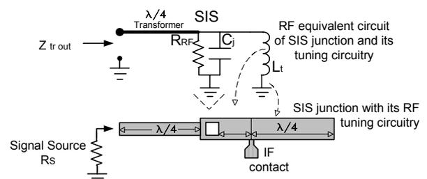
Fig. 9: Equivalent circuit of SIS junction and its tuning microstrip-based circuitry at RF. The impedance of the pumped SIS junction, R<sub>RF</sub>, connected in parallel with its geometrical capacitance C<sub>j</sub>. A piece of line acting as inductance, L<sub>t</sub>, grounded via λ/4 open stub, resonates C<sub>j</sub> at RF centre frequency. The impedance R<sub>RF</sub> is matched to the RF source impedance R<sub>S</sub> via a λ/4 transformer.
