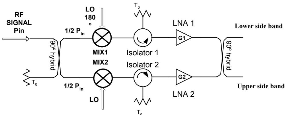
Fig. 1: Block diagram of the sideband separation mixer.
