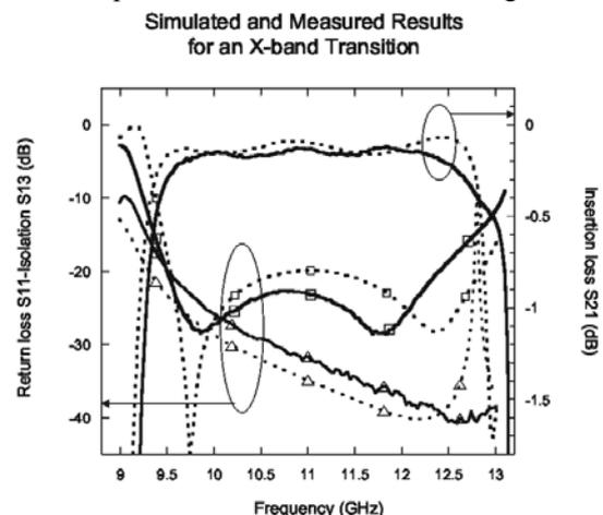
b) Measured and simulated results: upper curves are insertion loss, middle curves with squares are return loss and lower curves with triangles are isolation between RF and DC-IF ports.
