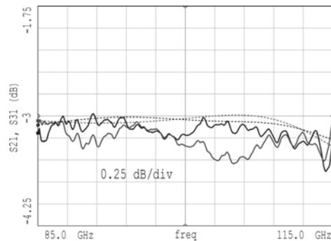
a) Waveguide to microstrip power divider as it was measured at 100GHz. The microstrip ports were replaced with microstrip to waveguide transitions. The waveguide is WG-10, the structure dimensions are  $S=340 \mu\text{m}$ ,  $W=95 \mu\text{m}$ ,  $L=270 \mu\text{m}$  and the substrate cross section is  $610 \times 150 \mu\text{m}$
