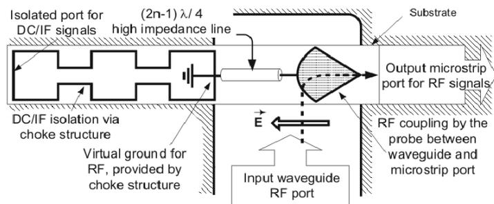
Fig. 4: The probe structure
