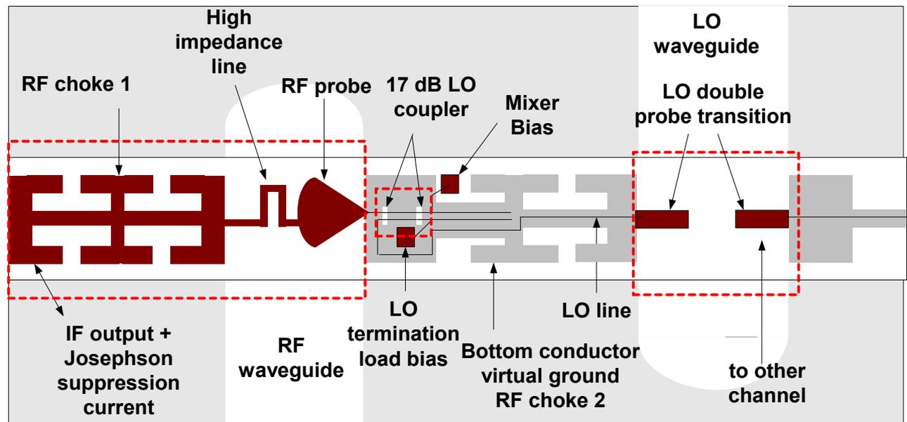
Fig. 3: Enlarged view of the left part of the 345 GHz mixer. Dashed areas indicate components that will be describe in more details in the next part.
